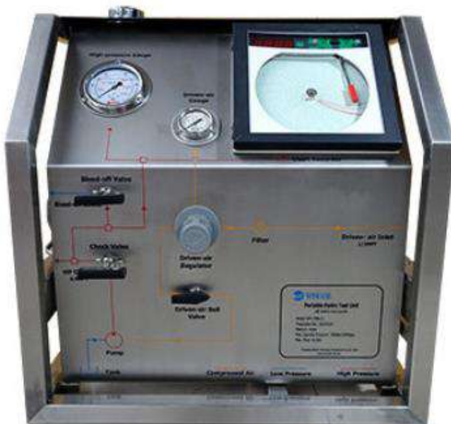
recorder for hydro test 500bar
